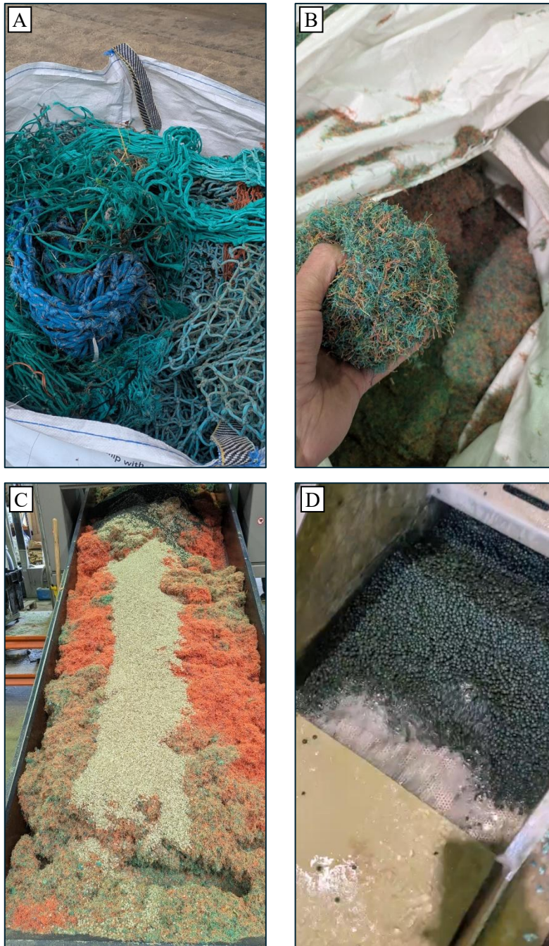
Figure 15: Processing of collected nets by Milspeed International Ltd. (A) Collected nets. (B) Shredded net. (C) Washing process. (D) Washing of pelleted net. Photos © Neil Hembrow, Ocean Recovery Project.
